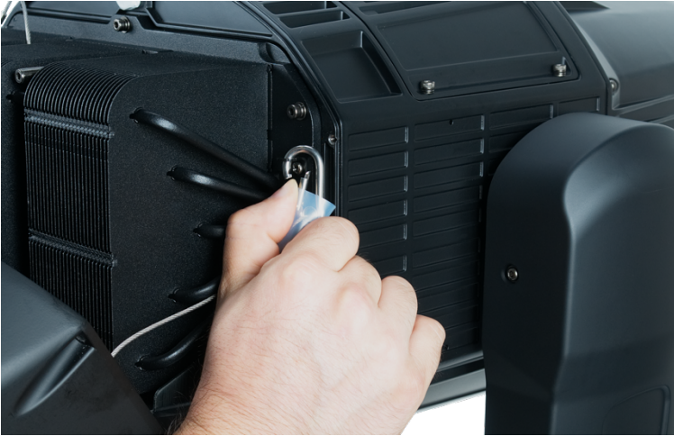
4. Unclip the rear cover safety cable.
