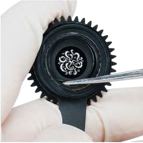
12. Carefully remove retaining spring.
