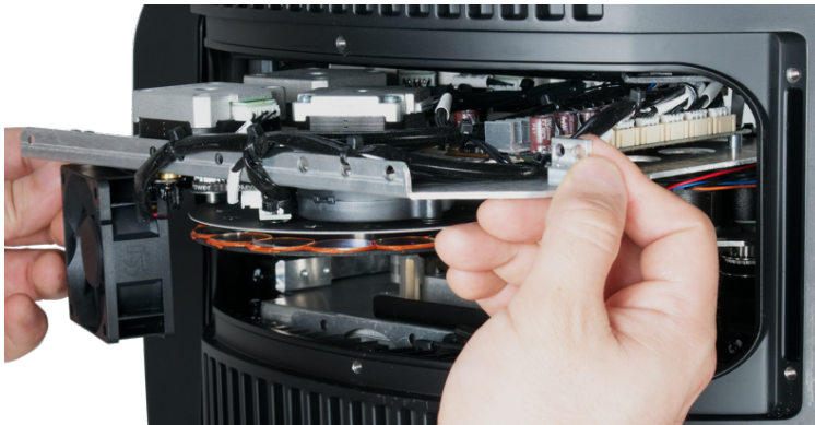
9. Carefully remove the effect module from fixture.
